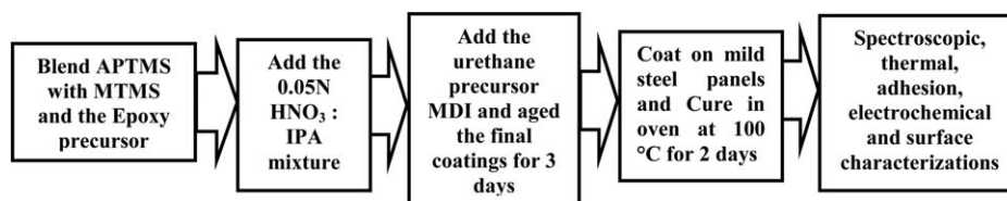
Scheme 1. Summarized process scheme for the development of the new coatings in this study.
